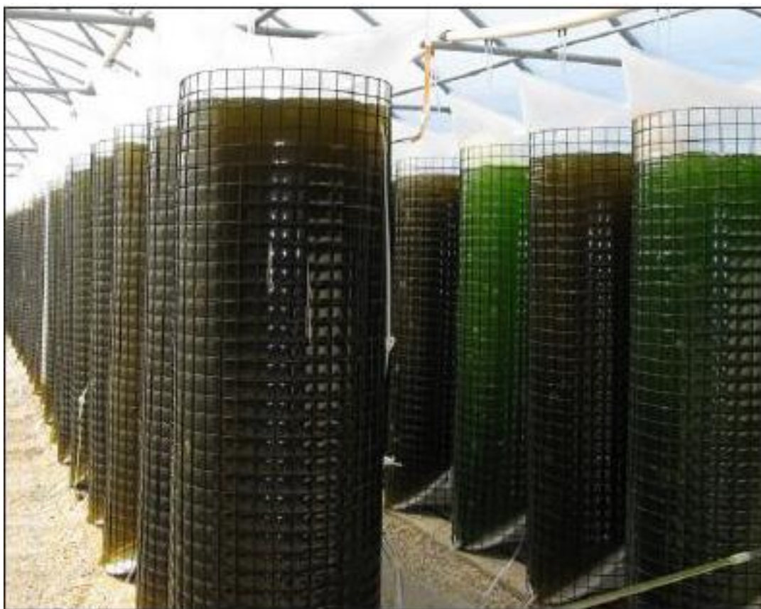
Polyethylene bags used for continuous culture of microalgae.
