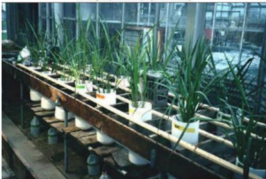
Figure 5. Zinc Uptake in Eastern gamagrass ( Tripsacum dactyloides ) Growing in Lysimeter Pots, Experimental Setup
